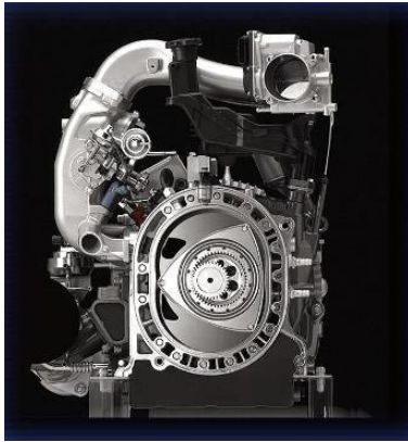
Fig.4 Cross-sectional diagrams of the hydrogen RE
